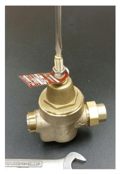
After loosening the lock nut, turn the center rod out (left) to reduce pressure.
